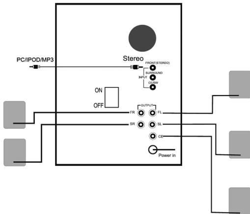
Step 1: Connect the device (PC/IPOD/MP3) to the Stereo Input Jack on the back panel with a 3.5mm stereo cable.
