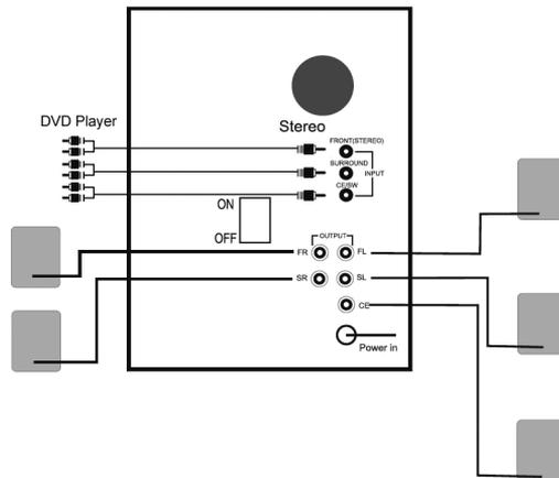
Step 1: Connect the device (DVD player) to the input Jack on the panel with 3.5mm Jack – RCA\*X2 cable X 3 pieces.
