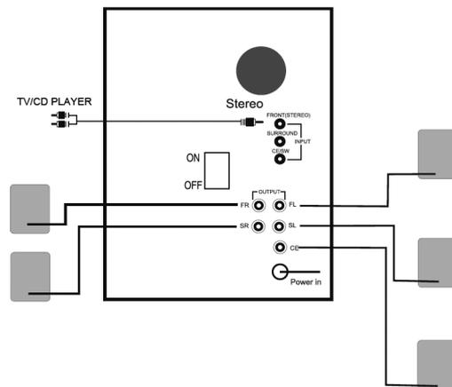
Step 1: Connect the device (TV/CD PLAYER) to the Stereo Input Jack on the back panel with a 3.5mm Jack – RCA\*X2 cable.
